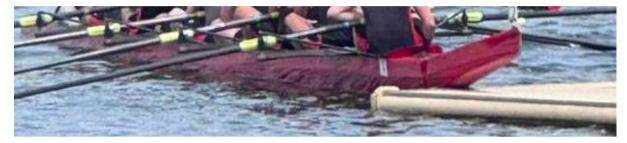
A Junior 8+ collided with an unmanned, partly submerged upturned dinghy floating down the river. The underside of the dinghy was black and would have been difficult to see. The fin and propellor of the dinghy caused considerable damage to the bow section of the 8+ and the boat will probably be written off. All crew members are thankfully unharmed, although highly shaken.
