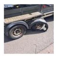
The damaged mud guard and wheel were removed by the driver, and the spare wheel fitted so that the journey could be completed.
